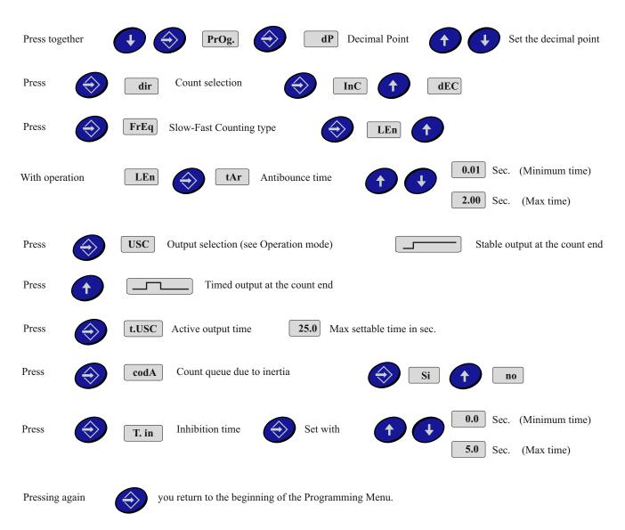
If after 5 seconds no operation is carried out, the instrument automatically exits programming, storing all the set parameters and the count digit appears on the display.
